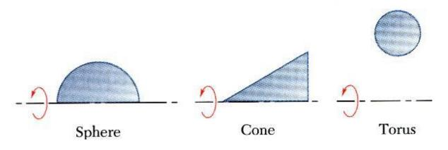
• Body of revolution is generated by rotating a plane area about a fixed axis.
