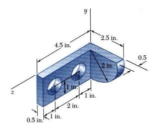
• Moment of the total weight concentrated at the center of gravity G is equal to the sum of the moments of the weights of the component parts.
