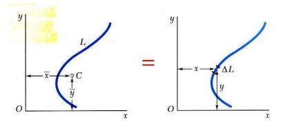
$\overline{x}W = \int x \, dW$   $\overline{x}(\gamma A t) = \int x (\gamma t) dA$   $\overline{x}A = \int x \, dA = Q_y$ = first moment with respect to y  $\overline{y}A = \int y \, dA = Q_x$ = first moment with respect to x
