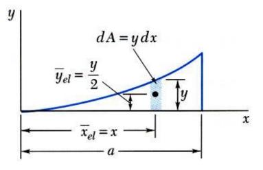
$$Q_{y} = \int \overline{x}_{el} dA = \int xy dx = \int_{0}^{a} x \left(\frac{b}{a^{2}} x^{2}\right) dx$$
