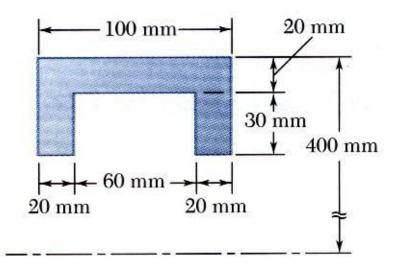
The outside diameter of a pulley is 0.8 m, and the cross section of its rim is as shown. Knowing that the pulley is made of steel and that the density of steel is  $\rho = 7.85 \times 10^3 \text{ kg/m}^3$  determine the mass and weight of the rim.
