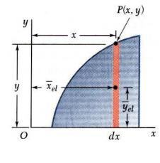
$\overline{x}A = \int \overline{x}_{el} dA$  $= \int x (ydx)$  $\overline{y}A = \int \overline{y}_{el} dA$  $= \int \frac{y}{2} (ydx)$
